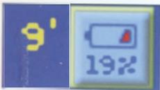
Once the minimum threshold of the working condition is reached, the residual operating time, indicated in minutes, is displayed besides the icon, surrounded by a flashing yellow frame.
