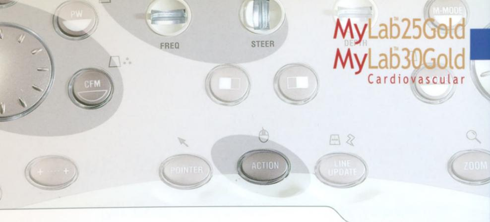
3. Activate the CFM ROI cursor by pressing the **ACTION** key to change the ROI size. The ROI can then be resized using the trackball.
