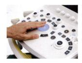
The layout of controls has been arranged to facilitate smooth operation, and a large palm rest at the center is designed to mitigate operator stress during examinations.
