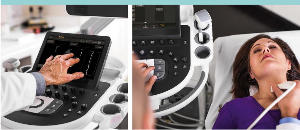
With image replication and TGCs on its tablet touchscreen, Affiniti 70 was designed to reduce reach and button pushes.
